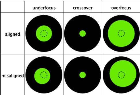
5. use the 2 mechanical adjustment knobs to shift the beam until there is no more lateral displacement going from underfocus to overfocus
